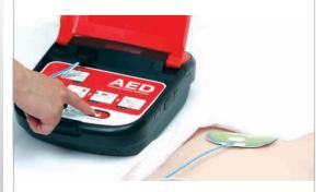
**3. PUSH THE SHOCK BUTTON.** Set the mode to adult or paediatric, then wait for the shock button to flash 'ready' for shock delivery. 1 COVER Protected icon sheet, shock button, adult/paediatric mode switch.
